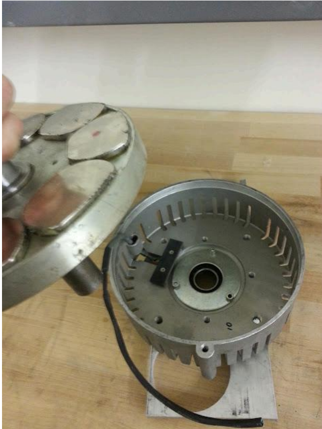
Ooh, the inside of the EtekMarsMotenergy Motor! And there's the sensorboard for the taking!
