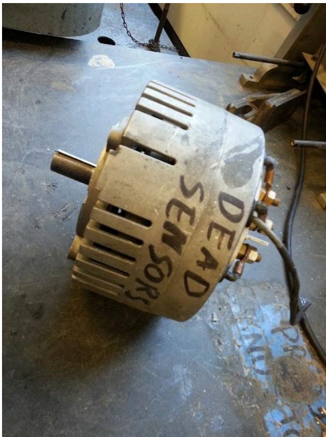
Meet the brushless Etek/Mars/Motenergy motor (EMMM? EM^3? EM3?). This one has dead hall sensors. How do I know?
