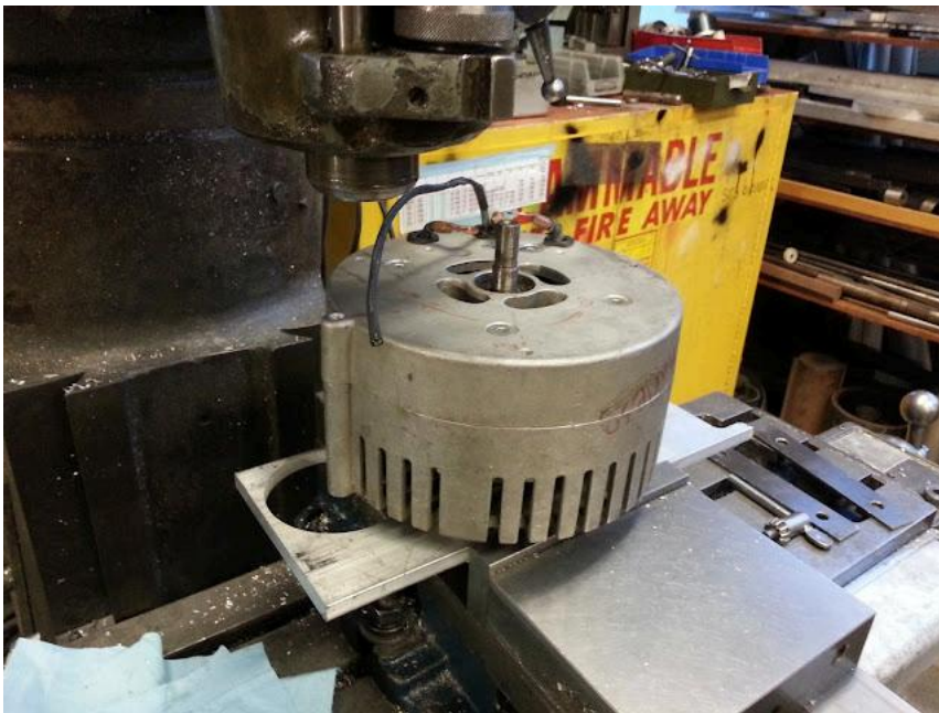
I mounted the motor on the mill on top of high parallels to allow the output shaft the room it needed.
