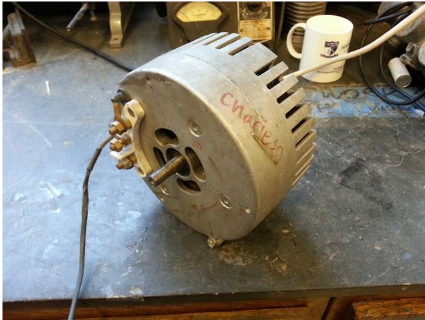
Meet the brushless Etek/Mars/Motenergy motor (EMMM? EM^3? EM3?). This one has dead hall sensors. How do I know?
